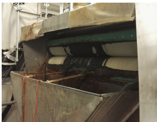
As pictured, drier material achieved with sonication concentrates on the middle of the belt. Before, the sludge was spread out all the way to the edges.
