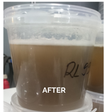
Before and after sonication: no visible dry material in the reject water after sonication.
