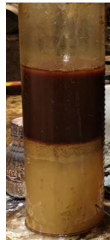
Before sonication: substantial amount of tall oil in the lignin removal
